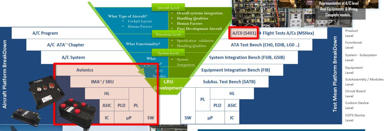
The V-Cycle can be decomposed in Intermediate Products ... and the Test Means Products needed to verify them
